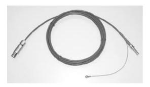
All HV cables now incorporate a new type of coaxial cable which uses Tefzel™ insulation, is rated at 15KVDC, is bakeable to 200 degrees C, contains a separate ground-sense wire and is radiation resistant.
